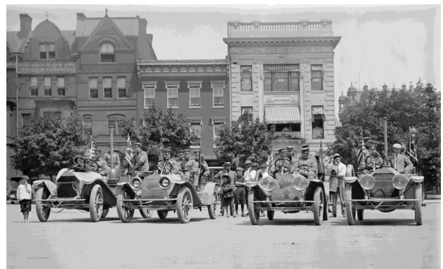
Photographed at a public event in 1911, two Balloon Destroyers are flanked each side by a Wireless Car. The right-hand Balloon Destroyers is the Academy's first Cadillac; it has been retro-fitted with a high-angle machine gun mounting. Note that the 1911 Model Thirty cars (the Wireless Cars) have larger wheels and tyres than the earlier cars. All tyres are treadless. (Harris & Ewing, 00372)
