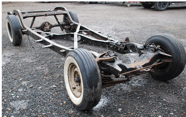
Refurbished 1950 Cadillac chassis
