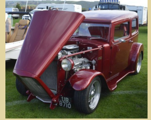
That '32 Standard 'Little' Nine with 350 Chevy motor, 700R4 Trans & 8" Ford Axle
