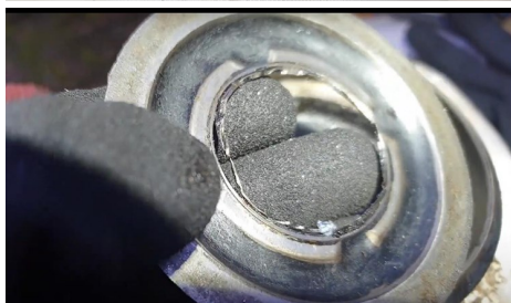
Close up of what the drive shaft was eating for lunch! Damaged oil retainer.
