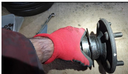
Rear wheel bearings were 'slack' and needed replacing.
