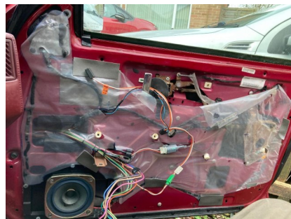
The next issue is getting to the lock mechanism. As you'll see there's a metal plate in the way. This holds the electric central locking actuator which operates on one of the four rods attached to the lock. It's riveted, so only option is to drill it out.
