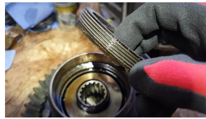
Last stage of disassembly... removing the gear retainer (after driving out a tapered locking pin).
