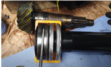
Another specialised tool. Pinion bearing puller..... and it made the job really easy. Worth the money.
