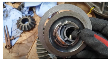
A bit of custom fab work needed to increase the diameter of the oil retainer to locate it 'central' in the bore and stop it from loosely wandering into contact with the driveshaft splines again
