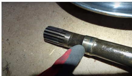
Nifty feature: There is a floating brass seal in the diff that mates with this sealing surface. I think, that together they act to the minimise oil loss from the diff into the axel housing.
