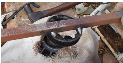
Who knew that you can 'weld' a race out of a blind bore? The heating softens and stress relieves the metal. Then the subsequent cooling shrinks it. It then becomes 'easy' to remove. Thanks YouTube! The only downside is it destroys the race!
