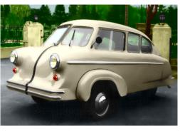
form an orderly queue. As a getaway car, it would be quicker by bus. The 199cc single cylinder 2-stroke engine produced 9.6hp at 4,900 rpm and 10.3 lb-ft of torque at 3,200 rpm. Weighing in at 380kg (that's 7.5 cwt in old money) it's top speed was 43 mph.
