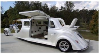
Built in 2012 by Wildlife -Tours of Australia, the Harley Davidson Limo bike is over 20 feet long and is powered by a rear mounted 5.7L 350hp Chevy V8 engine,. It has a bar, and seating for 8 people.
