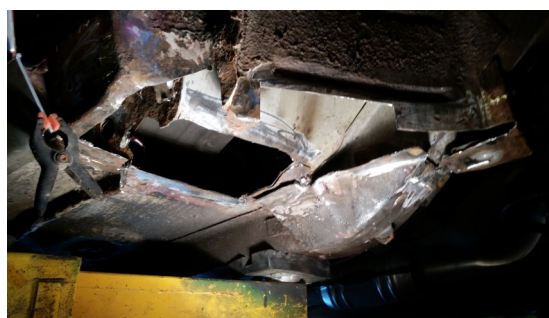
New metal being formed for welding
