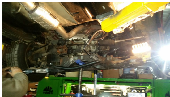
Rear sub-frame removed
