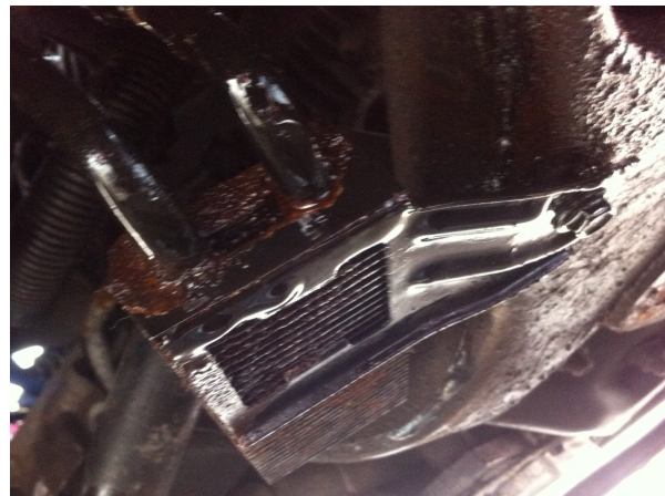
Leaking Power Steering Cooler
